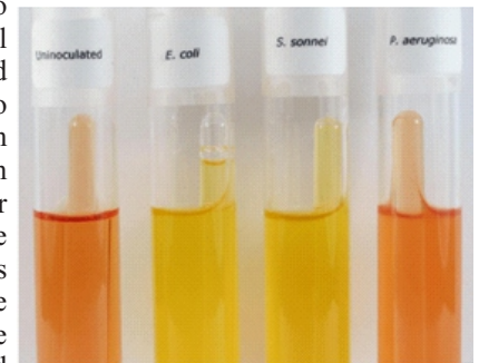
Figure 1. Peptone media with phenol red indicator. From left to right: Uninoculated tube; glucose fermenter with gas production (visible air bubble in the inverted Durham tube); glucose fermenter without gas production (no visible air bubble in the inverted Durham tube); non-fermenter.
