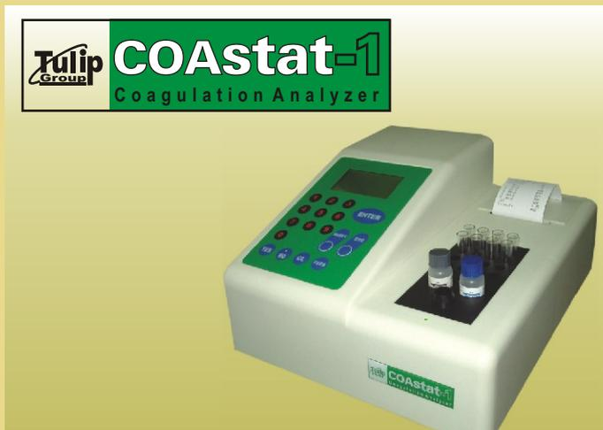
COAstat-1 is a single channel coagulation analyzer engineered with the ideal optomechanical measuring system. COAstat-1 operates with an automatic counter to trigger off as soon as the start reagent is added and stops the moment the clot is formed. COAstat-1 is suitable to perform all routine coagulation tests such as PT, APTT, TT, Fibrinogen, factor assays and clot- based assays.
